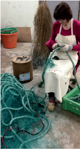
Brugte garn fraskæres til genmontering. / Old nets being cut off for remounting.
